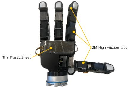
Figure 11: Friction modifications for Allegro Hand and ReSkin.
