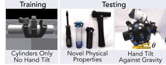
Figure 5: **Train and test sets.** We train with cylinders and no hand tilt in simulation. We test on real objects with varying COM, geometries, and hand angles. Motion capture markers on the objects are only for measuring task metrics.
